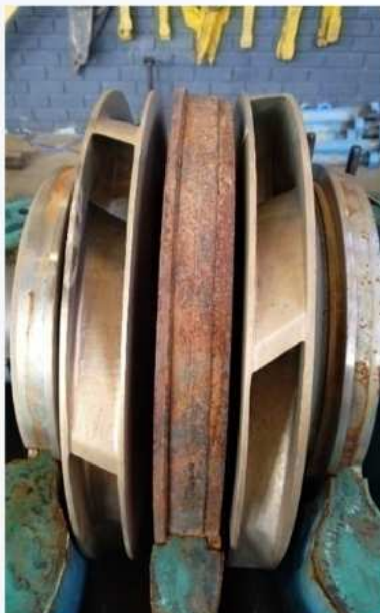
Stripping and assessing Secondary Pump 4
