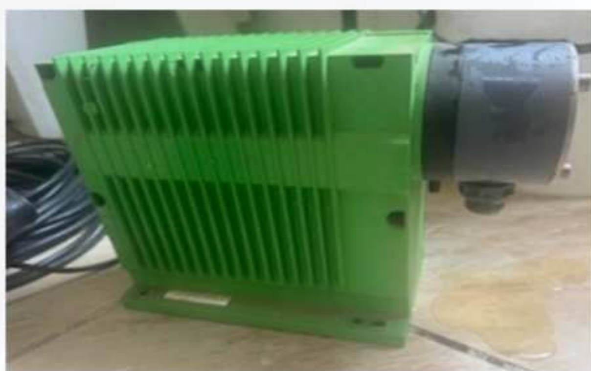
Old dosing pumps
